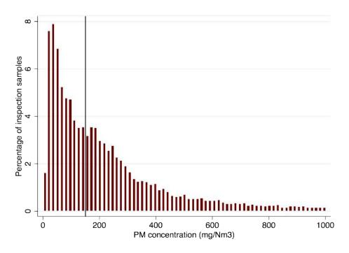
This histogram plots the number of samples from industrial plants in Maharashtra corresponding to various emissions levels, using over 13,200 digitized regulatory inspections data. While 150 milligram/Nm³ is the most common norm for particulate matter compliance, some industries have even more stringent limits. Source: MPCB and authors' research.
