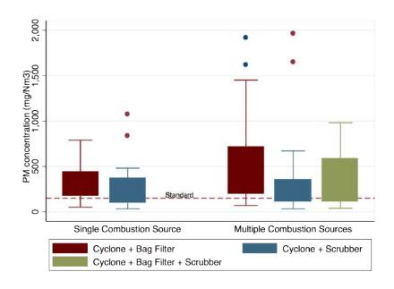
This boxplot shows the emissions of surveyed industrial plants in Surat with the most common pollution control equipment combinations. The box shows the interquartile range (25th percentile and 75th percentile), with the horizontal line showing the median. Source: Harish and Nilekani (2018).
