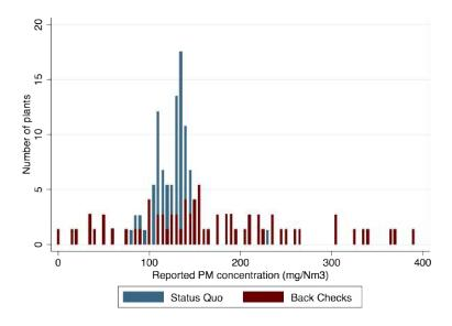
This figure shows the distribution of pollutant concentrations for particulate matter in stacks of control plants from audits and backchecks, during the midline survey of the project. The regulatory maximum concentration limit is 150 milligram/Nm³ (Duflo et al. 2013).
